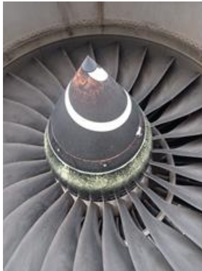
Figure 2 Erosion of the inlet cone due to FOD
