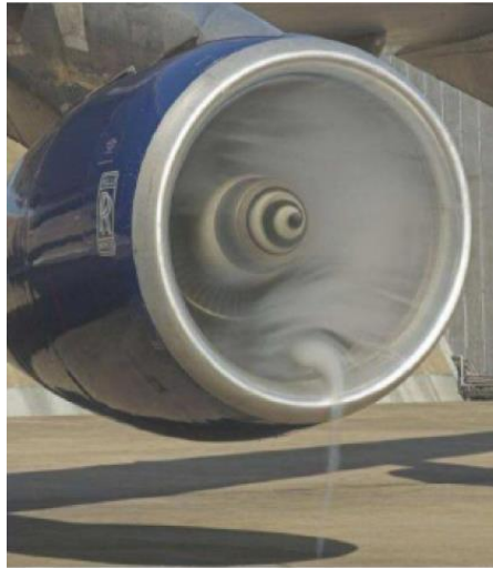
Figure 1 Ground vortex caused by ground idle of Trent700 engine
