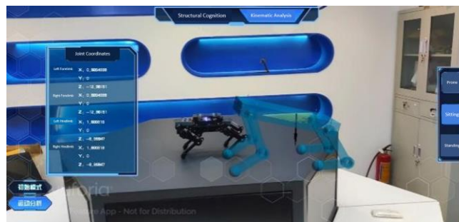
Figure 4: Real-Time Kinematic Analysis for Quadruped Robot.
