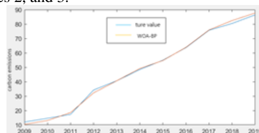
Fig. 3 Comparison of WOA–BP neural carbon emission predictions and actual values
