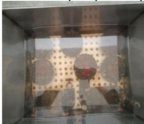
Figure 6: Constant temperature water bath immersion specimen
