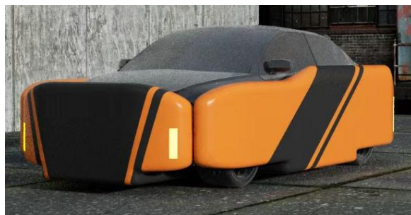
Fig. 1 Exterior design of the automotive anti-flooding device
