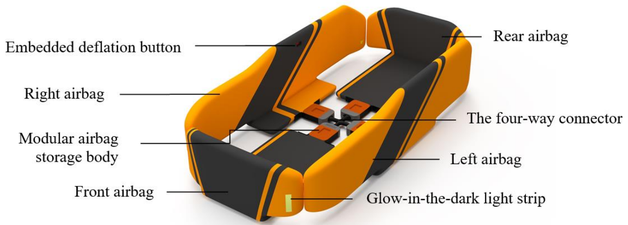
Fig. 2 Structural diagram of the automotive anti-flooding device
