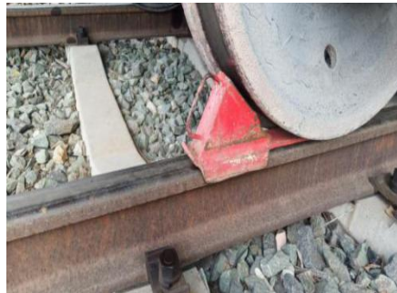
Figure 3a: Vehicles stored on a railway dedicated line are fixed with "iron shoes"
