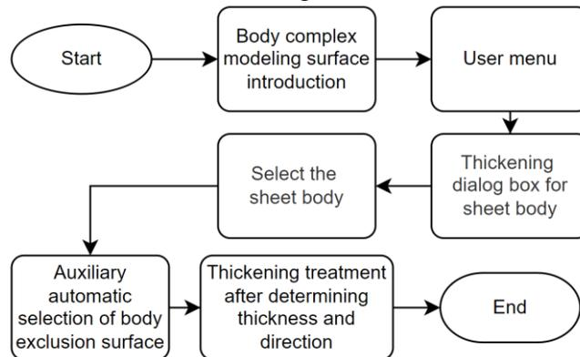
Figure 7: Automating thickening system workflow
