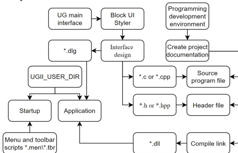
Figure 1: UG secondary development function system flow
