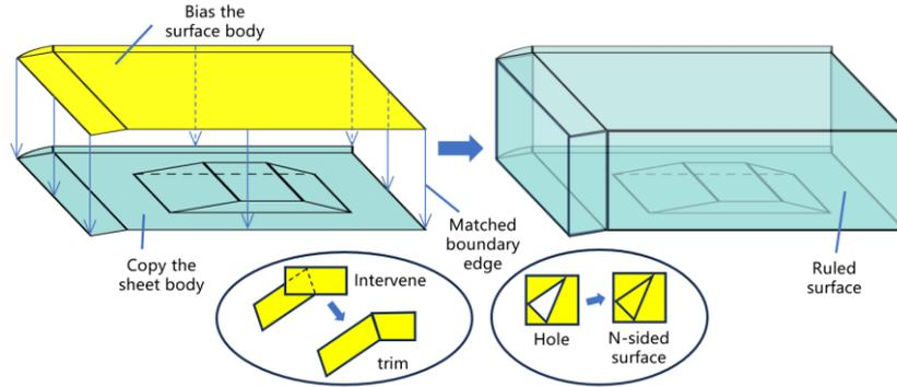
Figure 6: Sheet body thickening method
