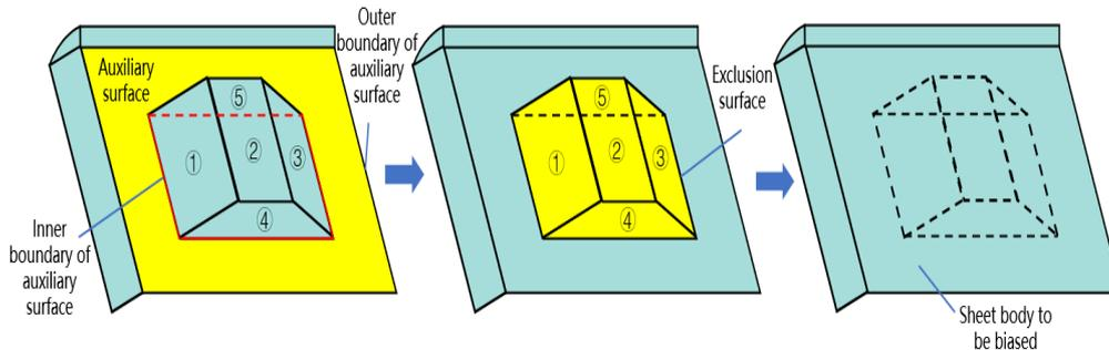
Figure 5: Auxiliary automatic selection of exclusion surface implementation method
