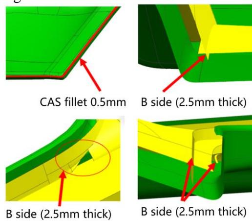
Figure 2: Part structure modeling thickening problem
