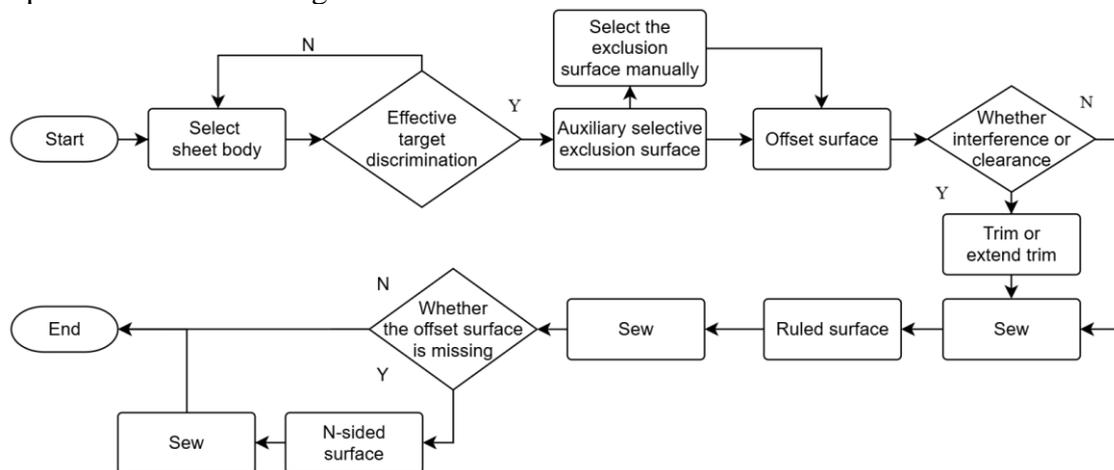
Figure 3: Automatic sheet thickening process
