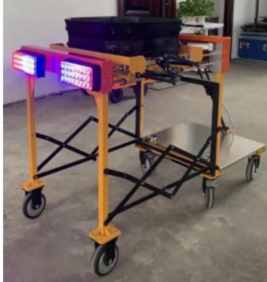
Figure 13: Traffic cone delivery car prototype
