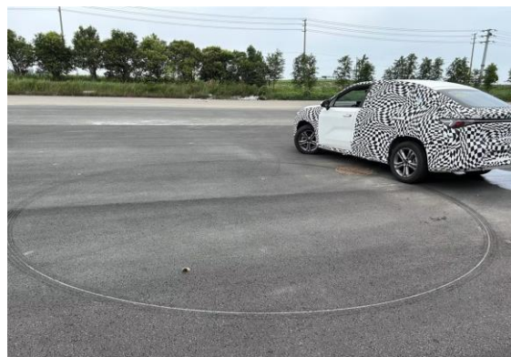
Figure 10: Trajectory with real vehicle testing of Braking the Inside Rear Wheel and the Minimum Turning Diameter
