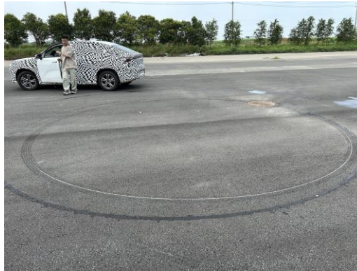
Figure 7: Real Vehicle Test Trajectory Diagram of Minimum Turning Radius without Control
