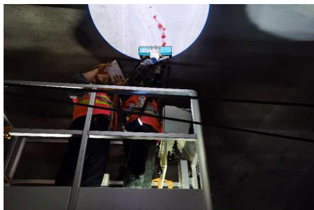
Figure 3: Field photos of ultrasonic detection of cattle farm slope tunnel
