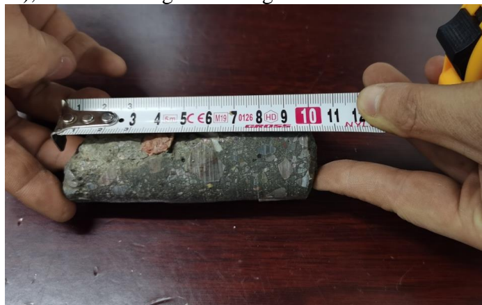
Figure 5: Measurement of the crack depth of the first set of drilling core sampling
