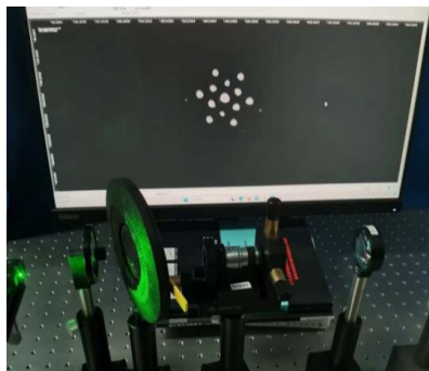
Figure 9: Measurement diagram of reciprocal lattice
