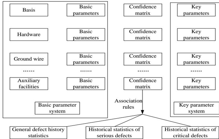
Figure 1: Overall process of constructing the key parameter system for transmission line status evaluation
