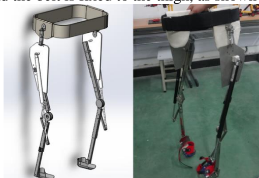
Figure 3: Lower limb fitness exoskeleton assembly diagram and physical picture
