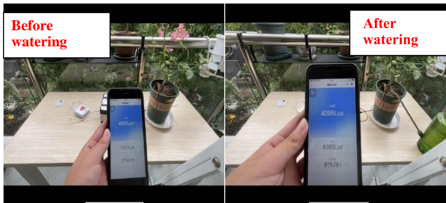
Figure 10: Program interface display before and after watering
