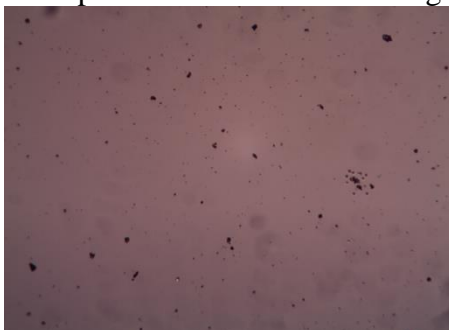
Figure 2: 400x optical microscope image of sodium lignosulfonate
