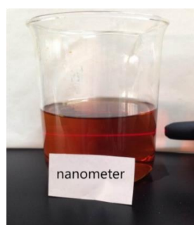
Figure 1: Tindal phenomenon of sodium nanolignosulfonate
