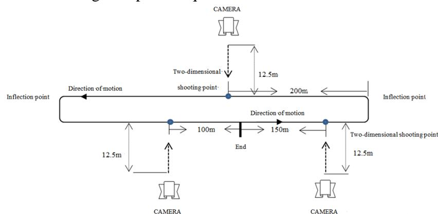
Figure 1: Schematic diagram of scene shooting layout
