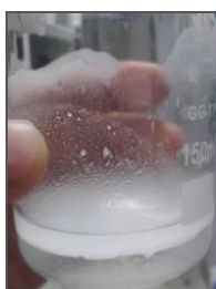
Figure 5: Macroscopic delamination of emulsion after gelation
