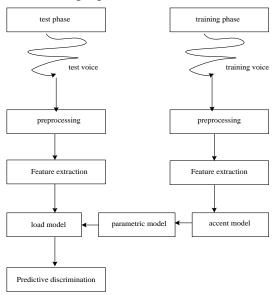
Figure 4: Spoken English CNN Model Recognition Architecture
