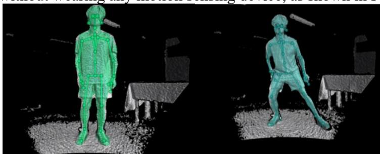
Figure 3: Kinect Obtain skeletal joint nodes
