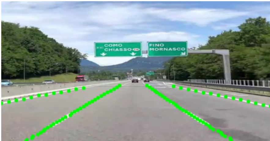
Figure 10: UFDL's lane anchor point recognition results for 4K resolution video sources
