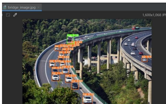
Figure 8: YOLOv8 recognition results using default pre-trained weights
