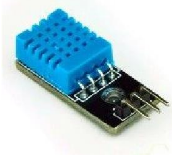
Figure 3: The sketch map of DHT11 temperature and humidity sensor
