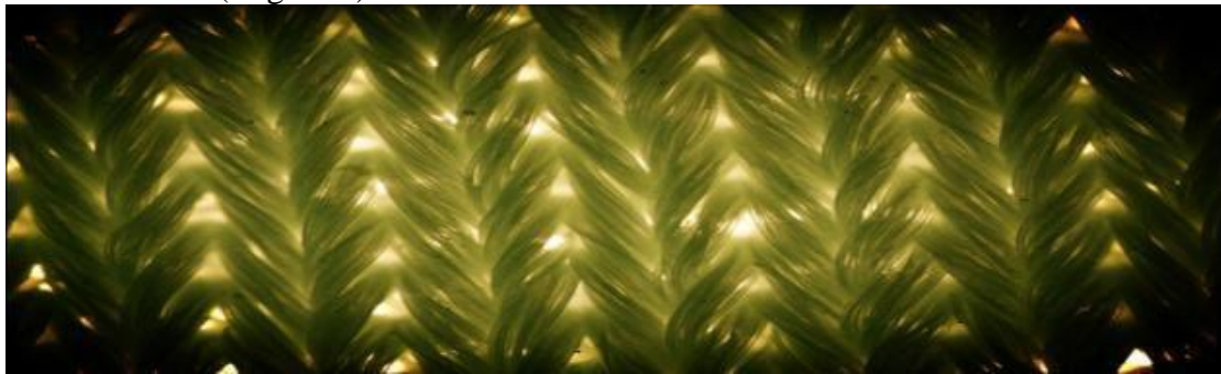
Figure 5: Cool Max under the microscope
