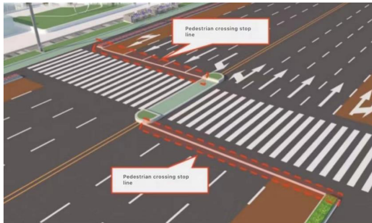
Figure 3: Schematic diagram of children friendly city crossing
