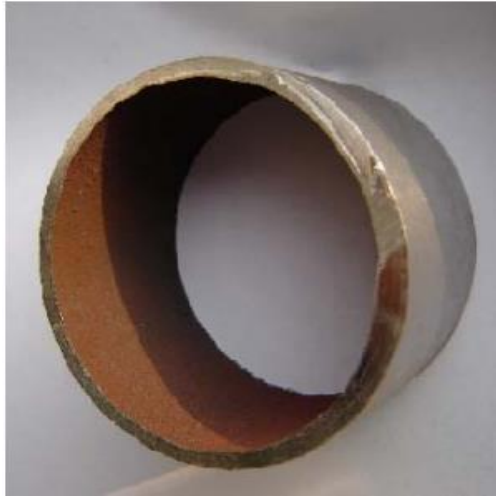
Figure 2: Inner surface of pipe section near window shaped bursting port.
