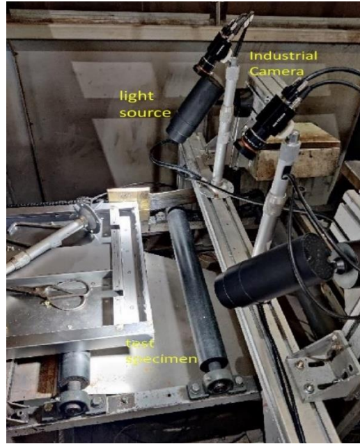
Figure 3: Welding spots defect image acquisition system
