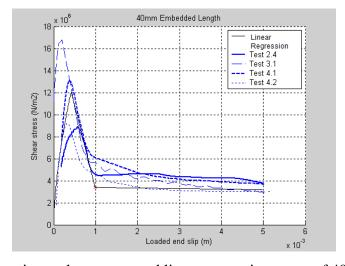
Figure: 38 (a): The experimental  $\tau$ -s curve and linear regression curve of 40mm embedded length specimens
