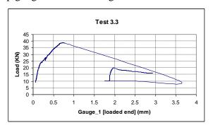
Figure 28: Load-Slip curve
