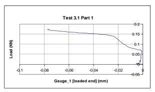
Figure 22: Load-Slip curve
