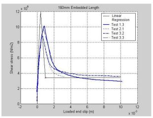
Figure: 38 (d): The experimental τ-s curve and linear regression curve of 160mm embedded length specimens
