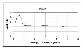
Figure 20: Load-Slip curve
