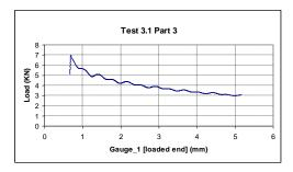
Figure 24: Load-Slip curve
