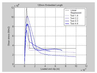
Figure: 38 (c): The experimental  $\tau$ -s curve and linear regression curve of 120mm embedded length specimens
