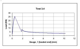
Figure 30: Load-Slip curve
