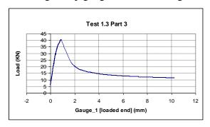
Figure 8: Load-Slip curve
