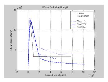
Figure: 38 (b): The experimental  $\tau$ -s curve and linear regression curve of 80mm embedded length specimens
