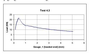
Figure 35: Load-Slip curve
