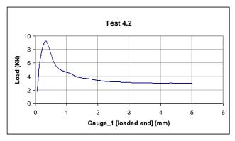
Figure 33: Load-Slip curve
