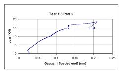
Figure 7: Load-Slip curve
