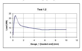
Figure 4: Load-Slip curve
