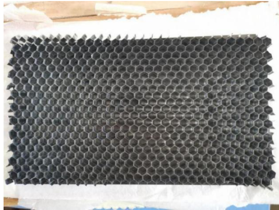
Figure 6: Sandwich structure of carbon fiber composite and aluminum honeycomb
