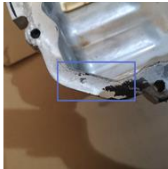
Figure 2: Oil leakage inspection of oil pan inspection
