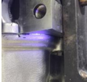
Figure 1: Oil leakage part
