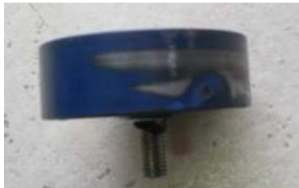
Figure 2: Figure of idler wear
