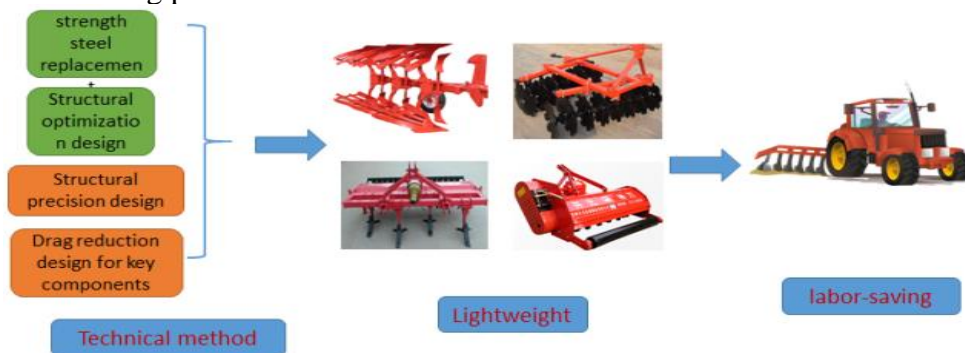
Figure 3: Lightweight of partial ground preparation machinery
