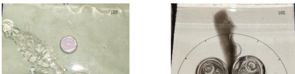
Figure 5 Deflection of gel under high pressure
