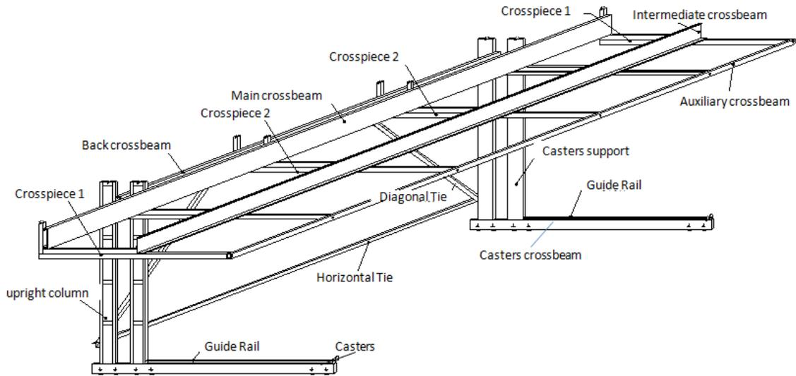
Figure 3: The stand Assembly without planking
