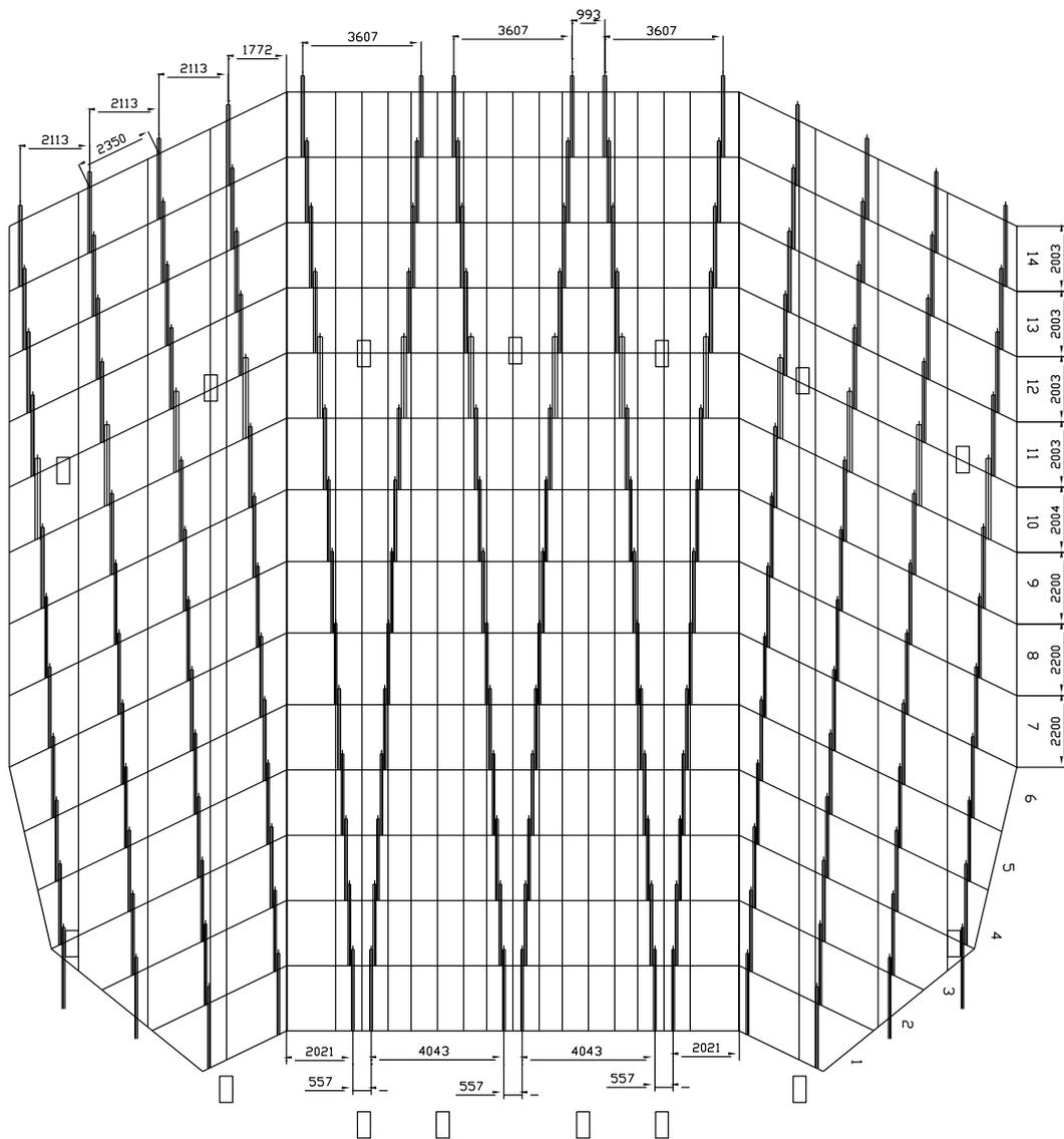
Figure 5: The distribution of support brackets for the grandstand countertops
