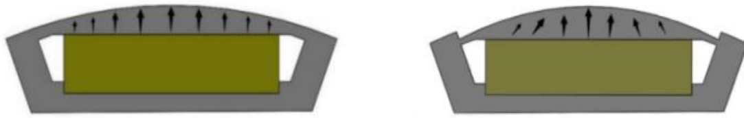
Fig.3 Comparison of rotor pole structure before and after optimization
