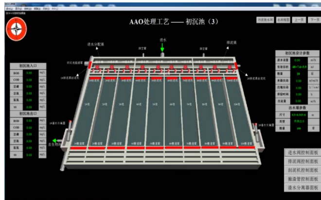
Figure 10: 2D primary sedimentation tank.
