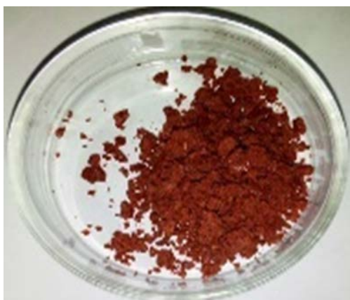
Figure 5. Fe-MOF obtained after synthesis and oven dried. It has a brownish colour.
