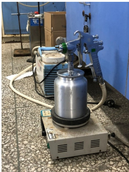
Figure 6 spraying platform. Emulsions are stored in the container attached to the spray gun, the white tube connects the spray gun with an air tank, which pressure is regulated by a pressure valve.
