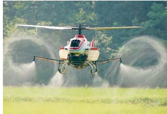
Figure 2 Accuracy of sprayed droplets are vulnerable to wind drift [9].
