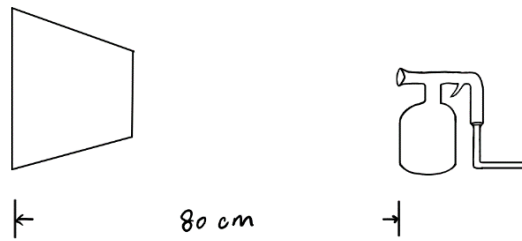
Figure 9 A simple sketch of arrangement of spray gun and target paper.
