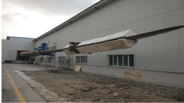
Figure 1: Wind turbine blade uniaxial resonance full-scale structure fatigue test.
