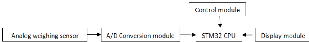
Fig.1 Hardware Design Diagram of Weighing System
