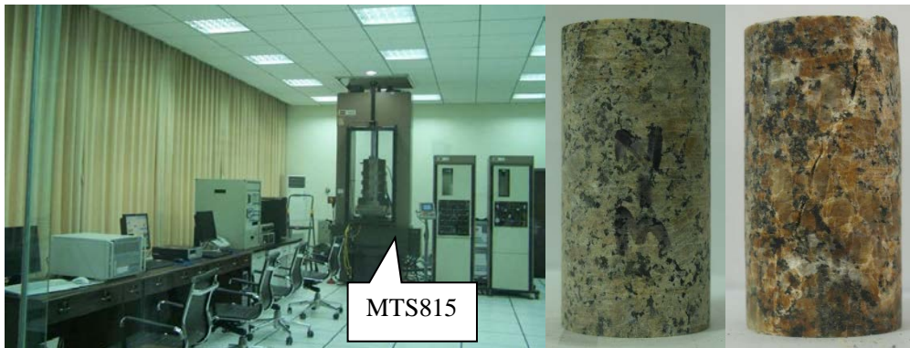
Figure 7: The test equipment and the samples of granite
