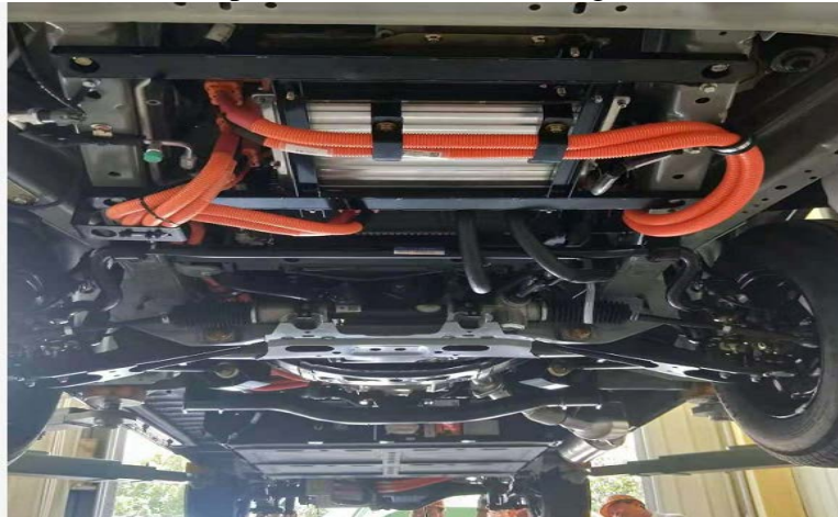
Figure 4: Chassis Range Extension Structure of Sample Vehicle
