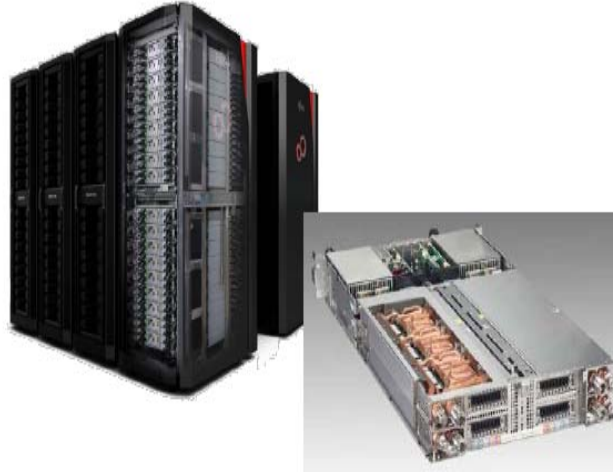
Figure 15 Fujitsu PRIMEHPC FX-100 Supercomputer
