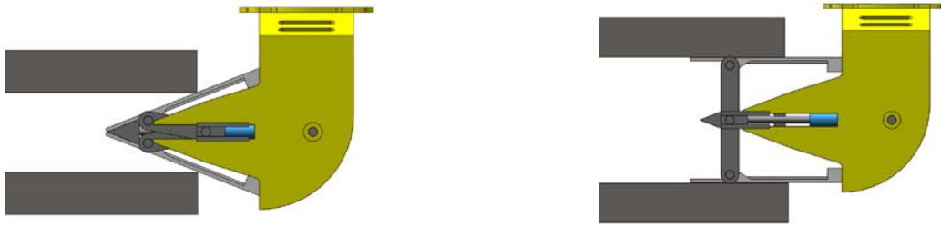
(a) Initial state of rescue attachment jacking process (b) Completion state of rescue attachment jacking process
