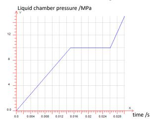
Figure. 7 Pressure loading curve of liquid chamber
