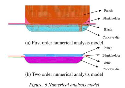
Using the sheet metal forming module in DYNAFORM, the thickness is set to 1.5mm. In the established model, all tools are regarded as rigid bodies and mesh. The structural material type is  $36 \times$  and the plate material is 4-node BT shell element. The three-dimensional digital analog grid is divided. The numerical analysis model is shown in Figure 6.
