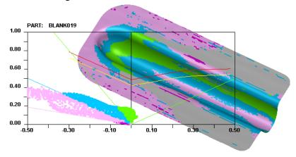
Figure. 9 Part firstly forming limit diagram (FLD)
