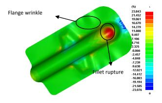
Figure. 5 Numerical analysis of rigid drawing
