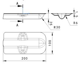
Figure. 1 Overall dimension of parts
