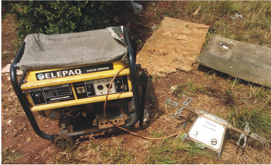
Figure 3: The flask shaker connected to the generator.
