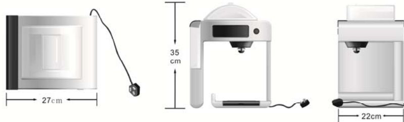
Figure 7 Dimension drawing of the coffee maker
