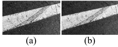
Fig.2.(a) Before median filter, (b) After median filter.
